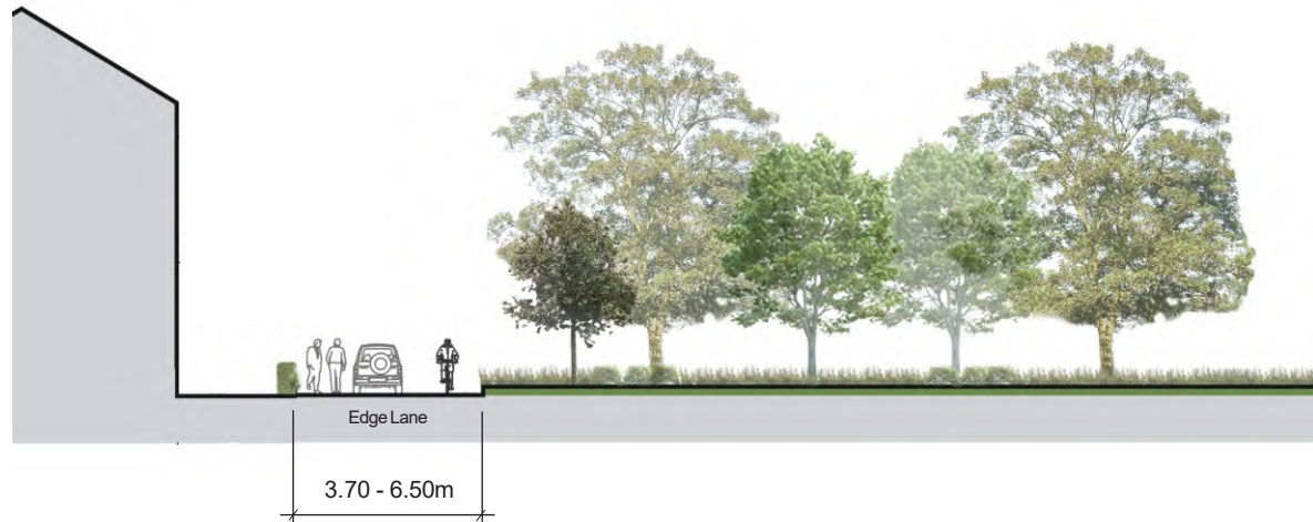
Figure 103: Cross-section to illustrate some dimensions for edge lanes.
