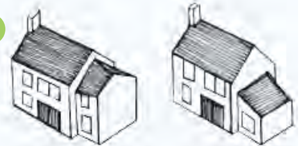
Good example for side extensions, respecting existing building scale, massing and building line.
