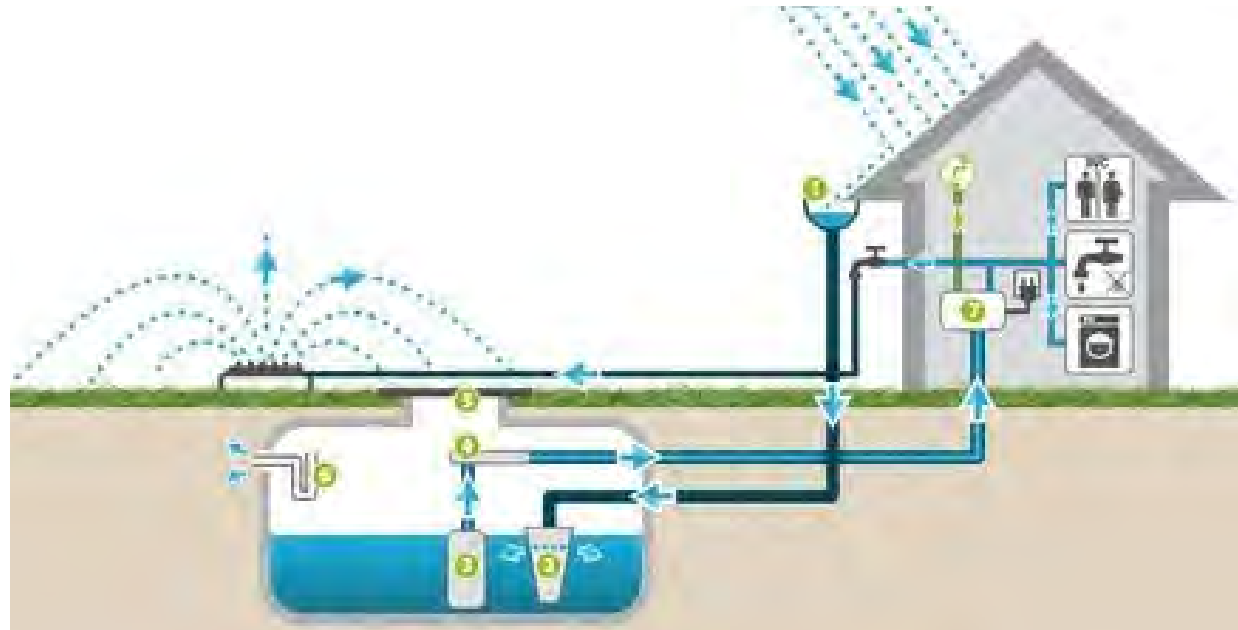
Figure 139: Diagram illustrating rainwater harvesting systems that could be integrated into open space and residential developments.
